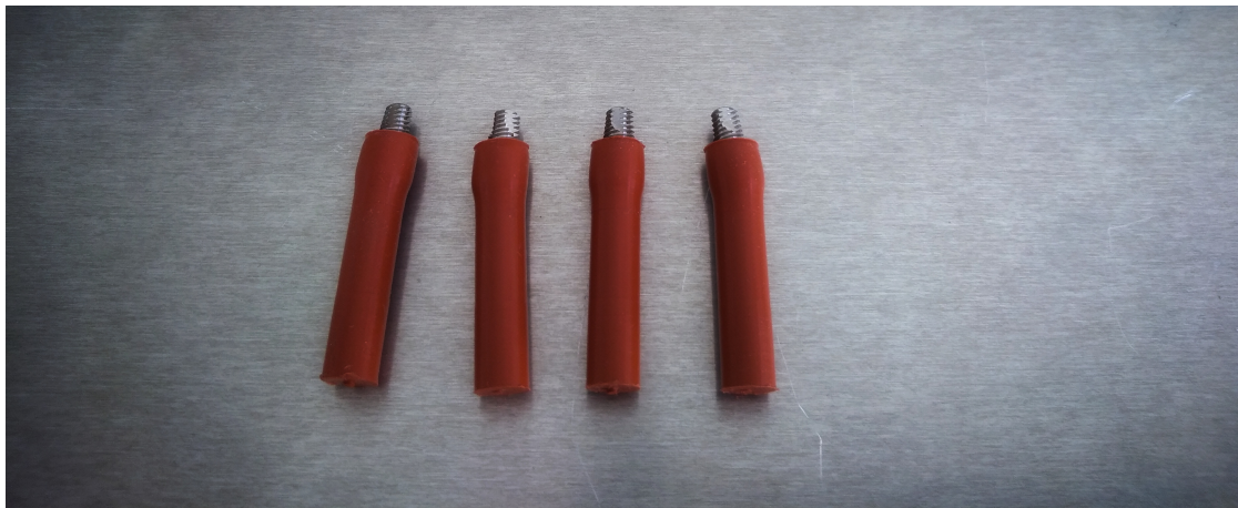
FIGURE 4.23: Image showing the samples before sand blasting
