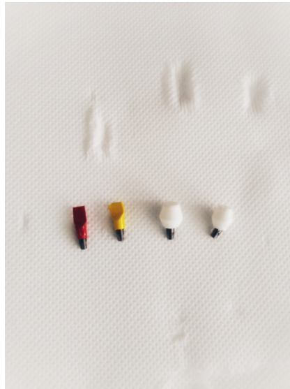
FIGURE 5.12: Dental implants after chemical treatment (without sand-blasting)
