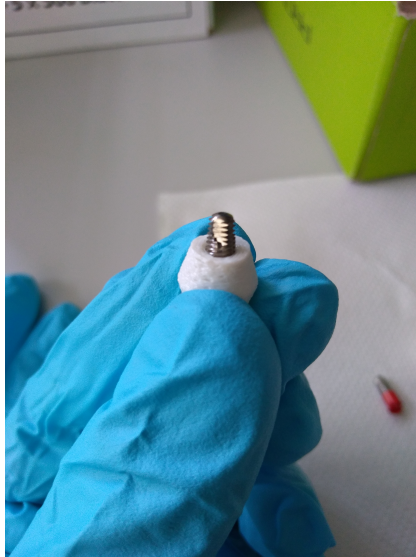
FIGURE 4.21: Image showing the 3d printed bio-inspired cap design 2
