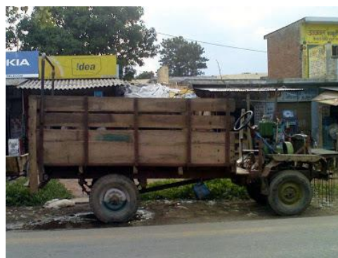
Fig.9 Jugaad vehicle powered by an agricultural water pump engine
