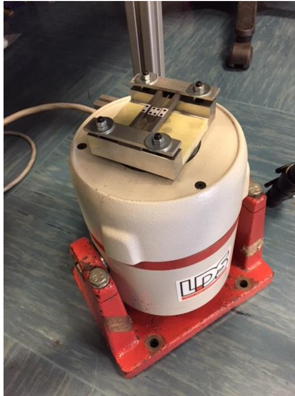
Figure 42: Electromagnetic shaker used for set 1 with sensor prototype equipped with the target on the rotor (internal centroids) and on the frame (external centroids)
