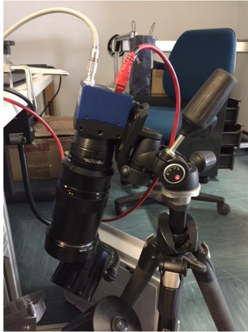
Figure 10: High-speed camera mounted on the tripod
