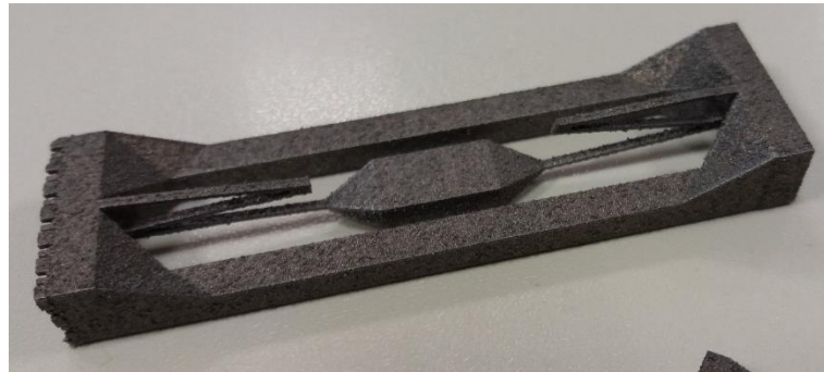
Figure 60: Sensor with different springs geometry used in set 2
