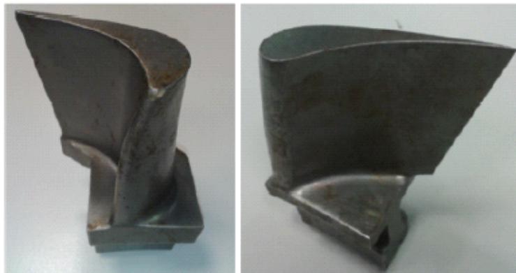
Figure 9.1: Rotor and stator blades.
