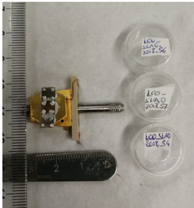
FIGURE 4.1: In this Figure we can see the sample holder preparation. From the top to the bottom, we have La_2CuO_4 with T_c = 22K , La_2CuO_4 antiferromagnetic - and thus insulating - and again La_2CuO_4 , but with a non measurable resistance, thinner than the others and ended with a larger Rocking Curve (Rocking Curve analysis reveals the broadening of the diffraction peaks - which is a way to evaluate the quality of the sample, see Section 2.3).
