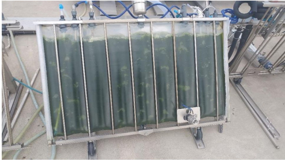
FIGURE 2.3.5.: FLAT PLATE PBR (WAGENINGEN UNIVERSITY, ALGAEPARC PILOT FACILITY) (ALGAEPARC, 2018)
