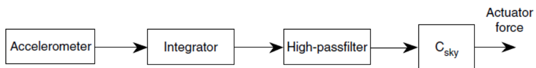
Figure 2.12 Practical implementation of sky-hook damping.
