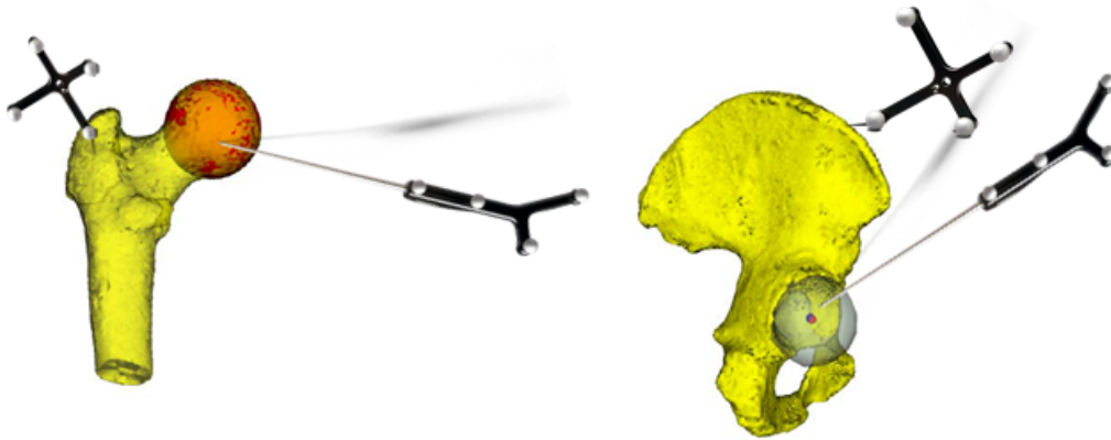
Figure 2.5: On the left, femur with DRF_f rigidly linked plus pointer tool. On the right, pelvis with DRF_p rigidly linked plus pointer tool
