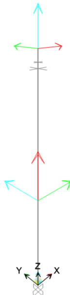
Figure 7.6: Model of a single bearing on SAP2000.
