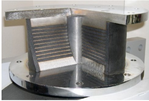
Figure 2.6: Cross section of a lead rubber bearing (adapted from Blanford et al. [2010]).
