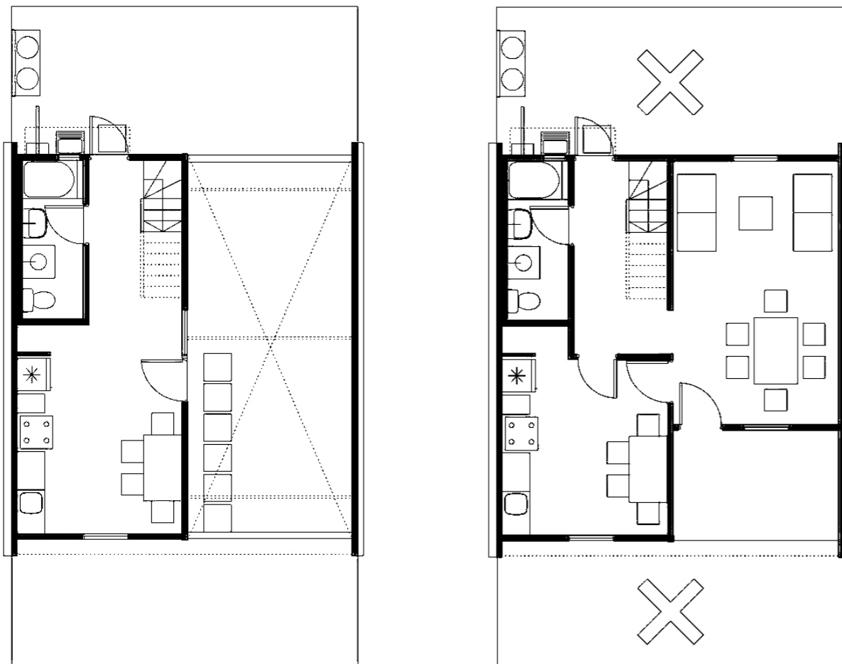
Figure 45. Villa Verde ground floor plan transformation (Alejandro Aravena, 2010)
