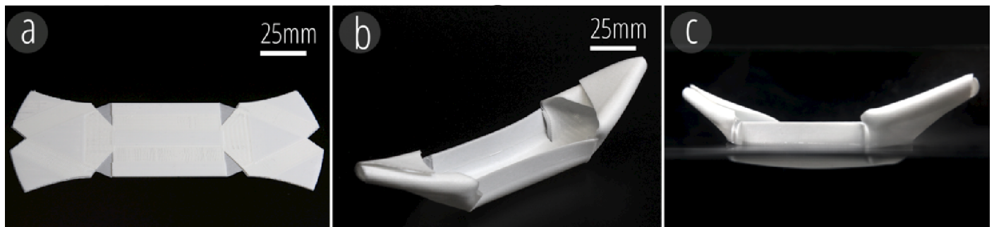
Figure 4.10 Self-folding boat: (a) a printed flat sheet (17.1x7.4cm); (b) a self-folded boat in 3D; (c) the boat can self-fold and float on a hot water surface.
