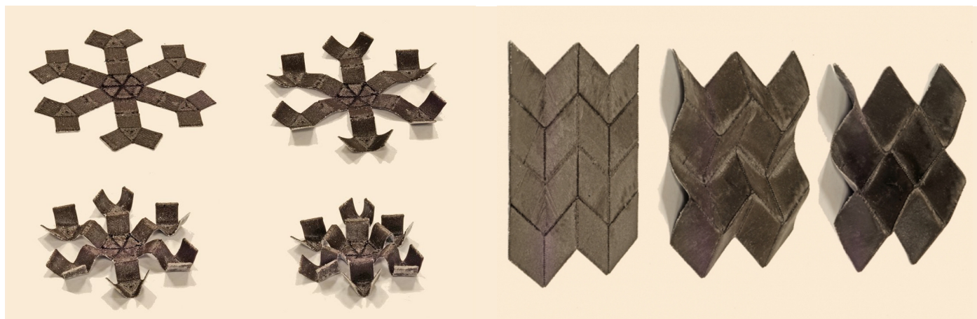
Figure 4.26 Different transformation of Spiderlike Grabber (on the left) and Miura-ori fold (on the right). Actuation of the demonstrated structures is performed by applying magnetic fields of 200 mT perpendicular to the planes of the structures.
