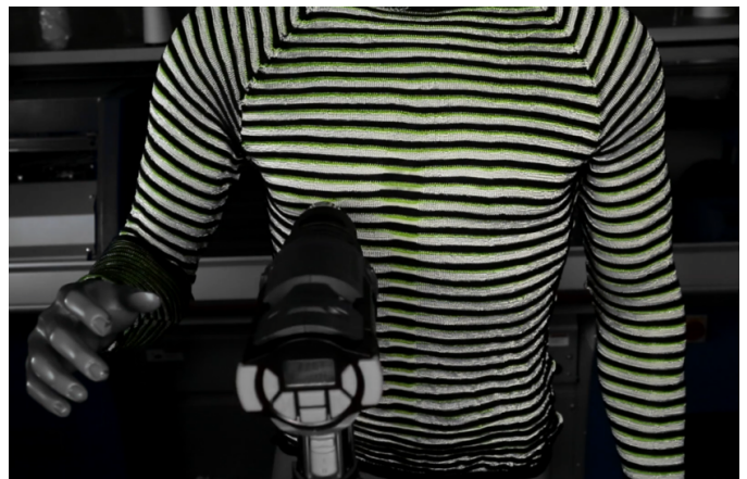
Figure 5.5 Demonstration of Active Textile that changes shape and structure in response to heat.
