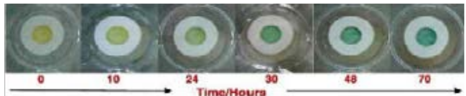
Fig. 48: Colour changes to a bromocresol green (BCG) sensor in response to a fish spoilage.. Source: Color Changing Plastics for Food Packaging By Lizanel Feliciano (Ohio State University)
