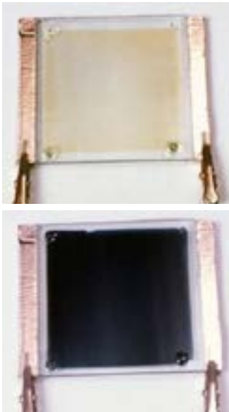
Fig. 42: Upper image: Here it's transparent and looks much like ordinary glass; Lower: Apply a small voltage and it turns opaque (blueish and dark). Source: photos by Warren Gretz courtesy of US Department of Energy/National Renewable Energy Laboratory (DOE/NREL)
