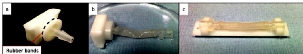
Figure 5.3: Mounting procedure for the scaffolds. (a) The POM assembling tool is used for helping in the anchoring of the scaffolds on the 1/8" barbed male slip luer connectors through rubber bands. (b) Once the scaffold fits the connector, the rubber bands are released on it. (c) When both the ends of the scaffold are anchored to the connectors, it is moved in a POM holder.
