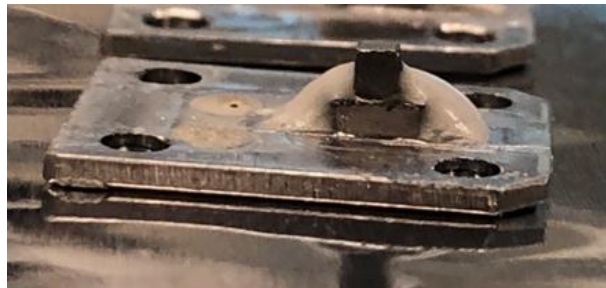
Figure 4.4: Picture of a \text{YFe}_2\text{Al}_{10} mounted on a sample holder for knife cleaving. The glue is covering the sample to fix it, the top part of the sample is left with no glue to allow the cleave.
