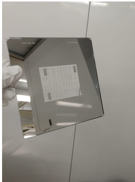
Figure A.5: Image of a typical quartz photo-mask used in our clean room.
