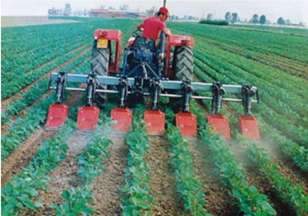
Figure 2.2: Inter-row rotary cultivator for inter-row weed control (Tornado, 2011).
