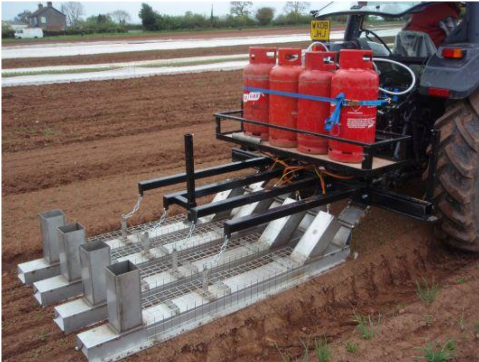
Figure 2.10: A crop-row flame weeder using LPG gas to control weeds inside the crop row (Physical weeding, 2011).
