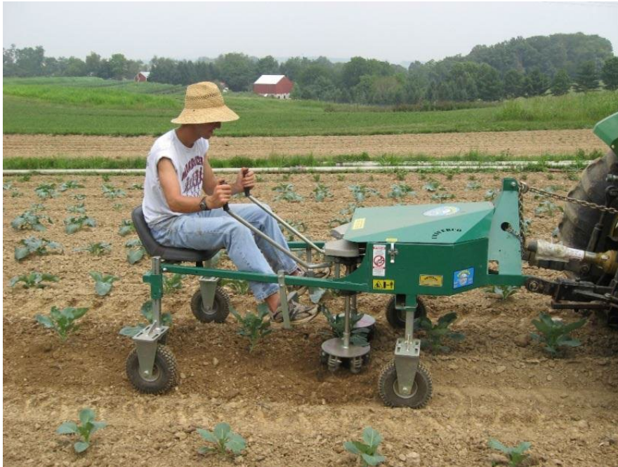
Figure 2.7: ECO weeder uses rotating weeding mechanisms with tines (Hillside Cultivator Company, 2011).
