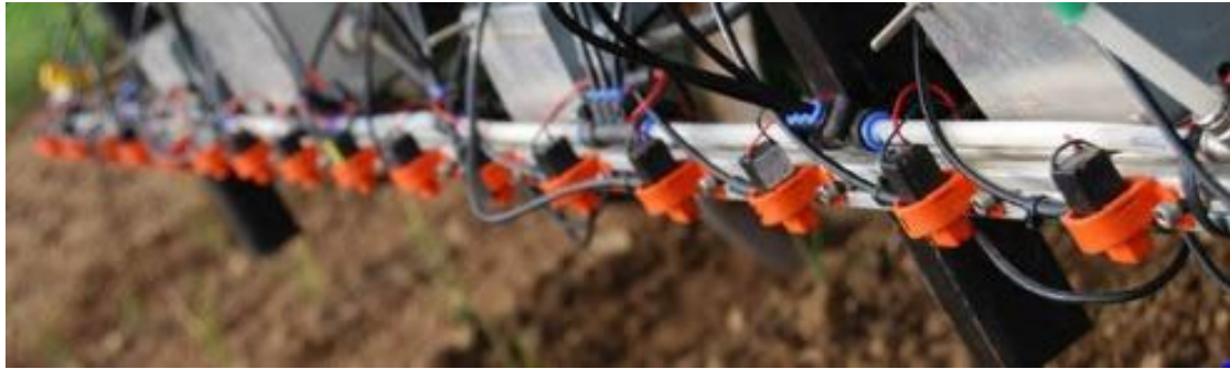
Figure 2.9: Intra-row chemical weeder with fixed nozzles
