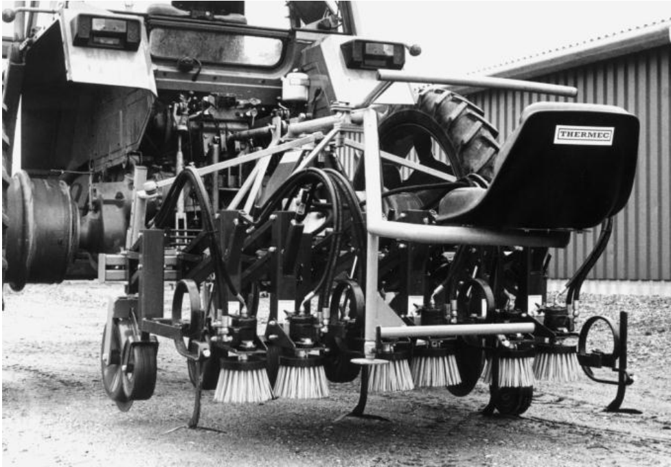
Figure 2.6: Vertical-rotating brush weeder use hydraulics and require an operator to control the brushes (Melander, 1997).
