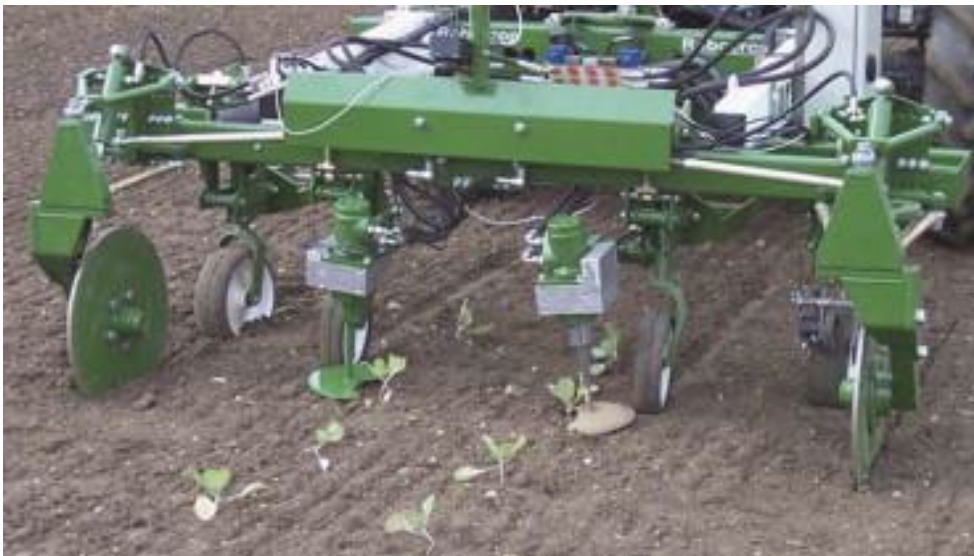
Figure 2.12: Automated weeder machine using hydraulics to rotate semi-circle discs that are used for weed control (Tillett et al., 2008).
