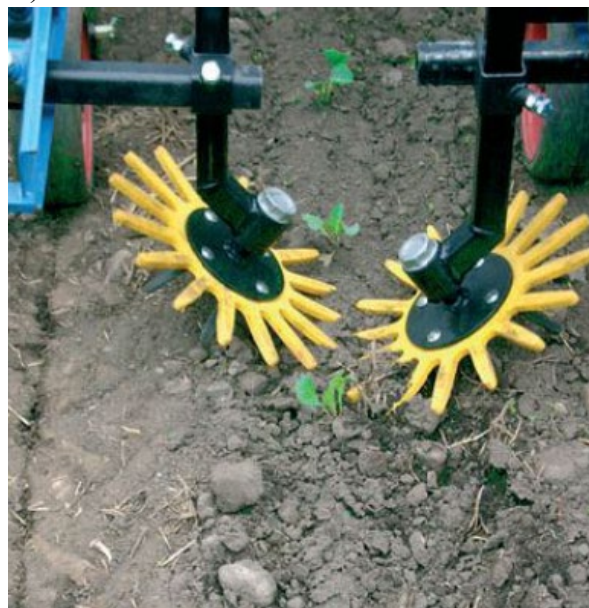
Figure 2.4: Finger weeder uses rubber spikes that are pointed at an angle towards the crop ( weide et al., 2008).
