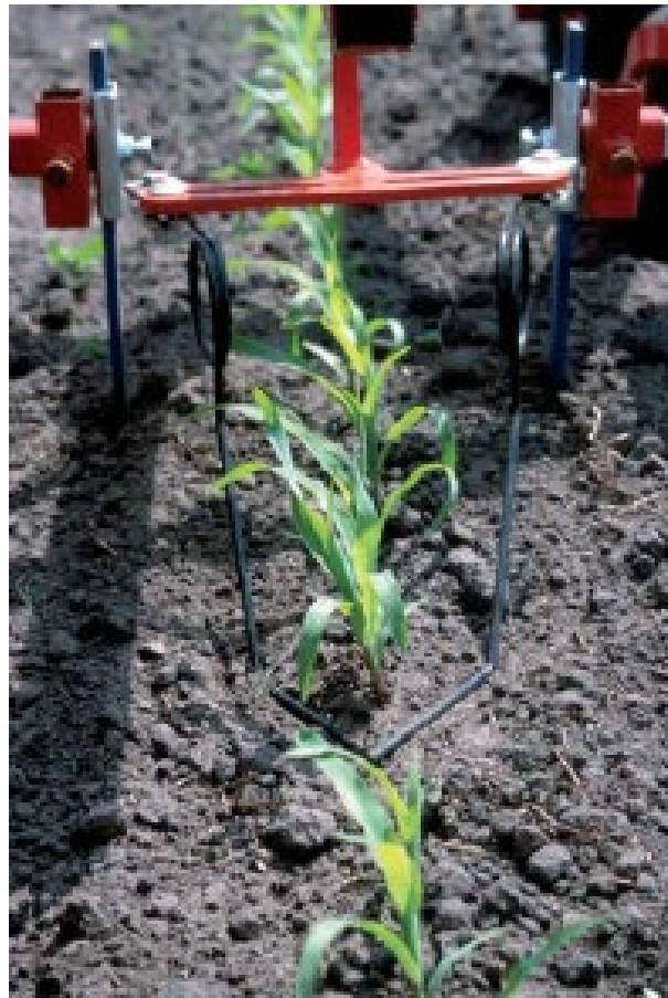
Figure 2.5: Torsion weeder uses flexible coil spring tines to sweep the weeds ( weide et al., 2008).
