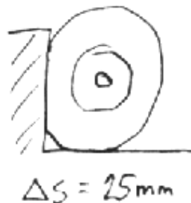
Figure 4.18: Deformation of the tyre, when hitting an obstacle with 1 m/s.
