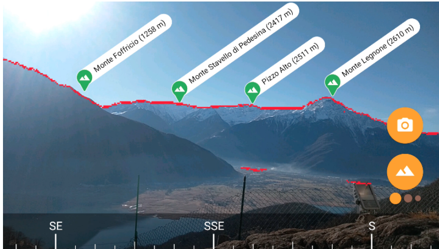
Figure 2.8: The skyline extracted from the computer vision module from the frame of Figure 2.7.
