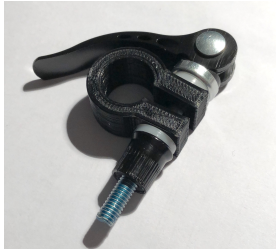
Figure 4.13: Carbon fiber tubes locking mechanism.
