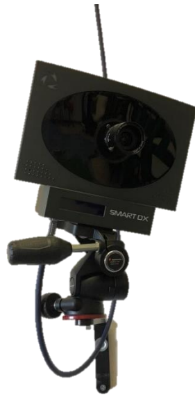
Figure 15-Camera of the motion analysis system, equipped with LED crown.
