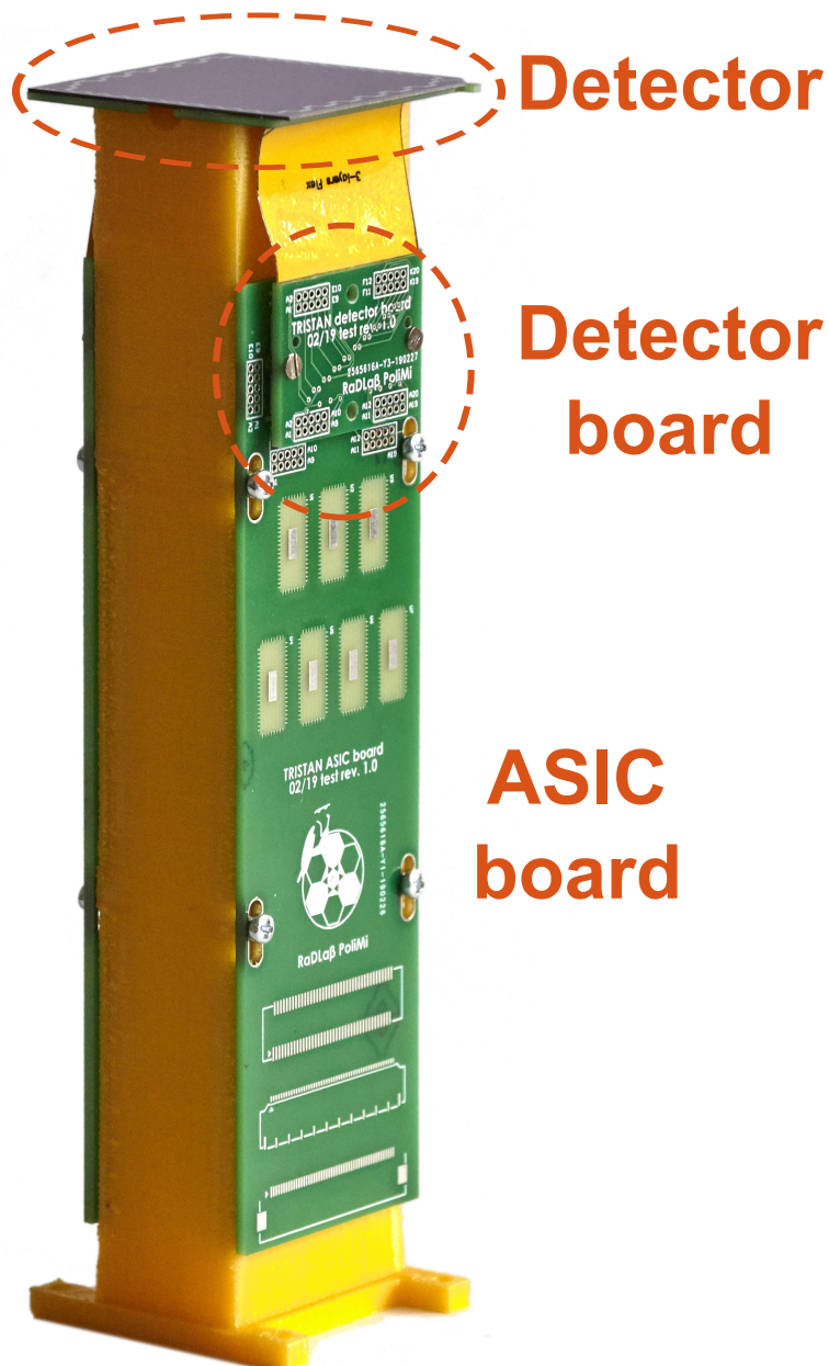
Figure 1.21: Target design of a single module in TRISTAN. We can see the detector on its corresponding board and the ASIC board with the space needed to bond the ETTORE's chips.
