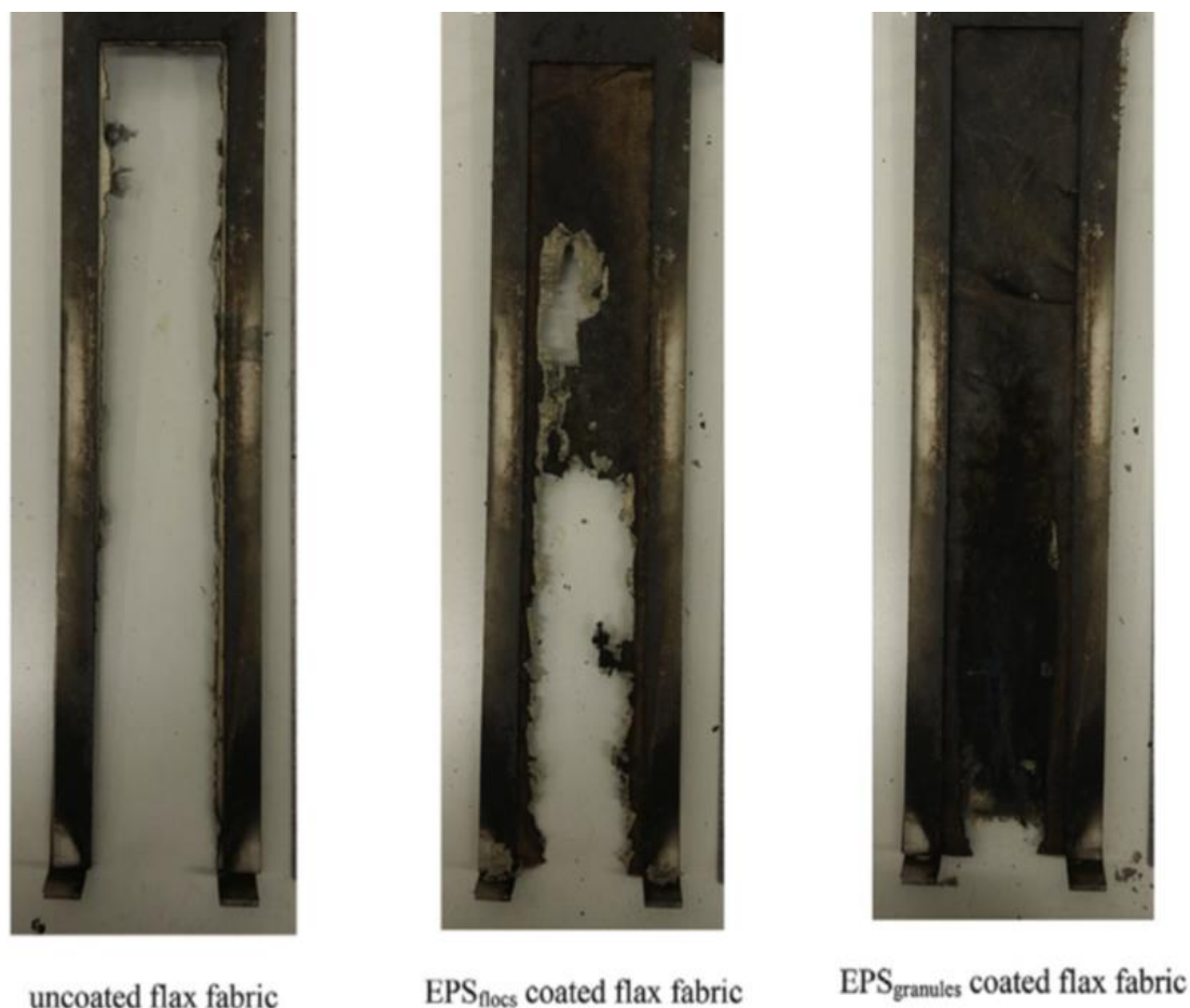
Figure 10 Comparison between uncoated flax fabric, EPS flocs coated flax fabric and EPS granules coated flax fabric after burning for twelve seconds, respectively (Kim et al. 2020)
