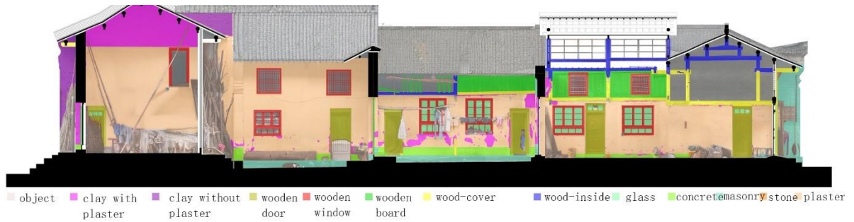
Fig. 5.4 Material of section B-B in May 2018 (Elaboration by author according to ICOMOS-ISCS)
