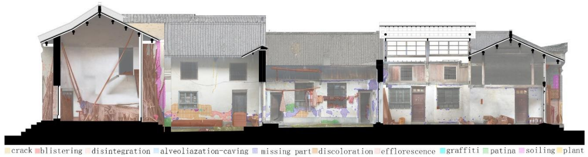
Fig. 5.5 Decay of section B-B in May 2018 (Elaboration by author according to ICOMOS-ISCS)
