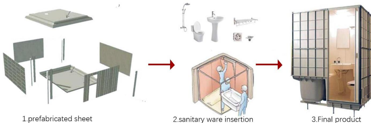
Fig. 2.29 Installation flow chart of the integral toilet (Source: Fu Fei, 2019)
