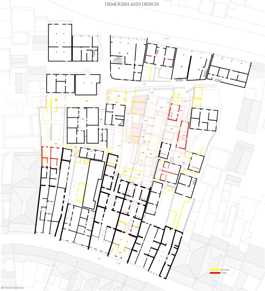
Fig.4.8 The demolish and design of the aera (Elaboration by author)
