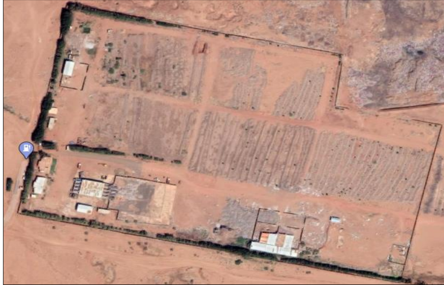
Figure 12: The figure shows the premises of the Omdurman landfill including the cells, offices, sorting facility, composting pad and plastic recycling plant. Source: Google.
