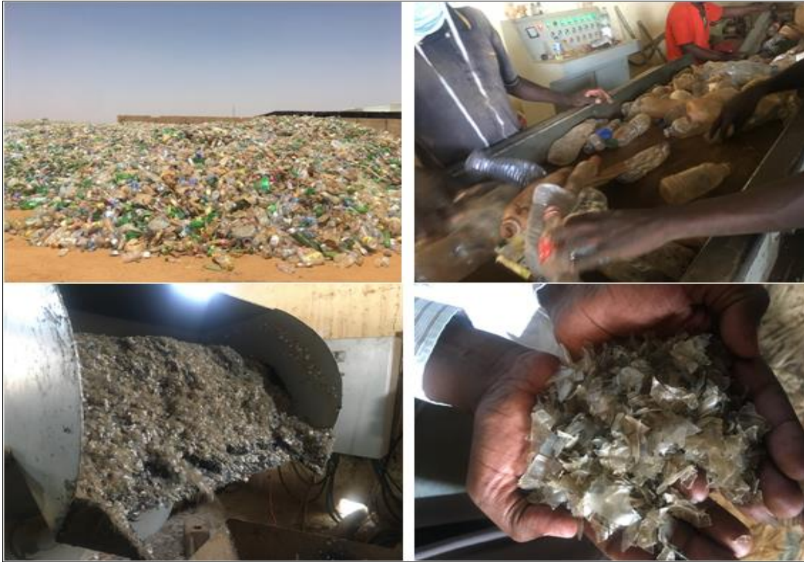
Figure 14: The PET plastic recycling facility showing the receipt area, the manual sorting line, grinder and the finished product.
