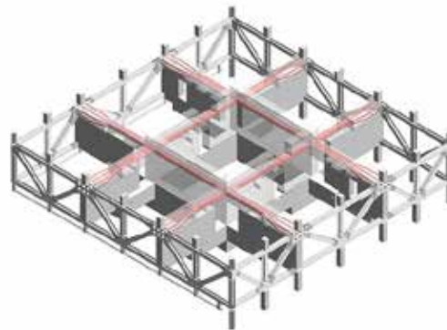
Fig. 05.6 -Post tensioning truss system
