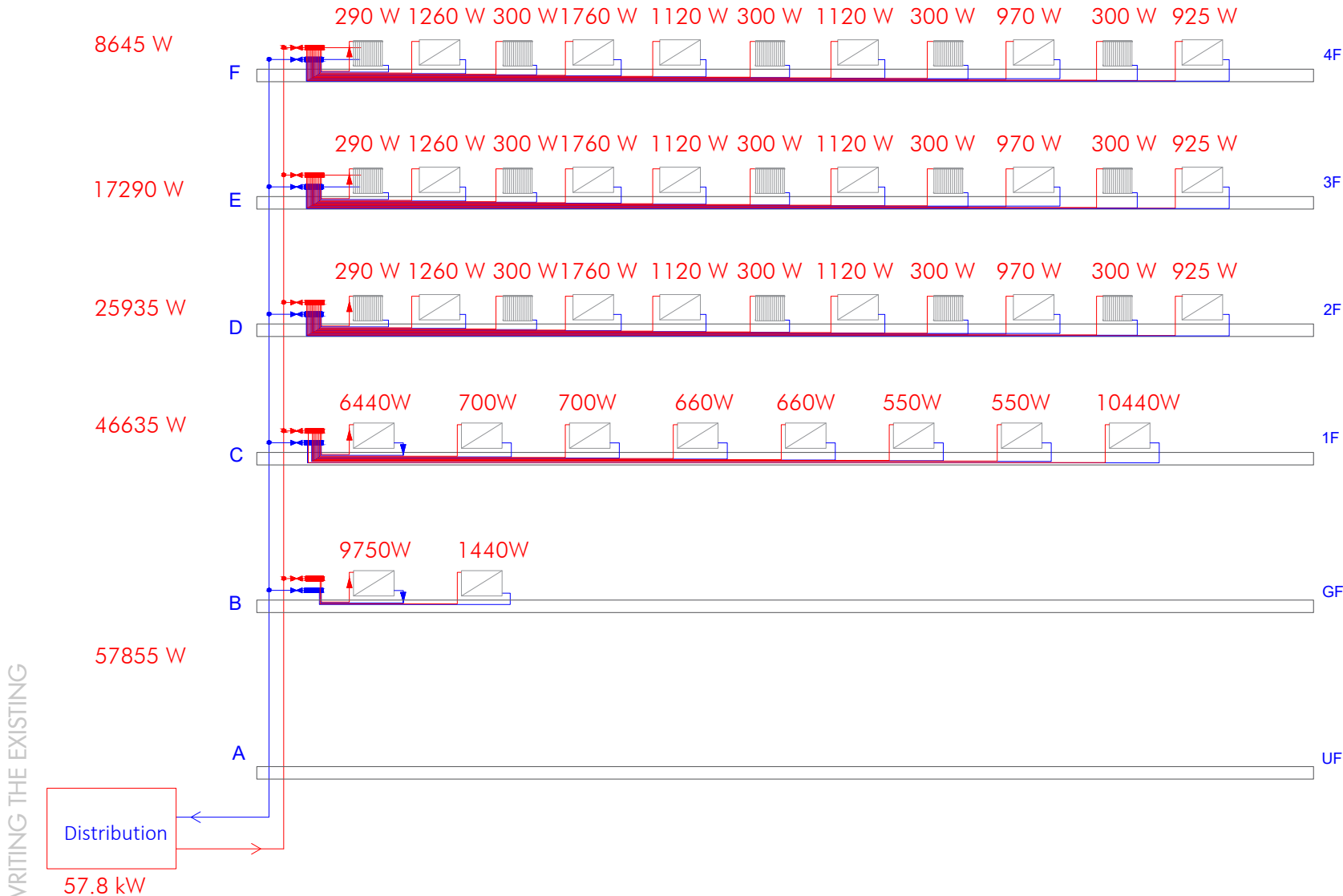
Fig. 05.44-East wing heating system scheme and partial plan 1:200
