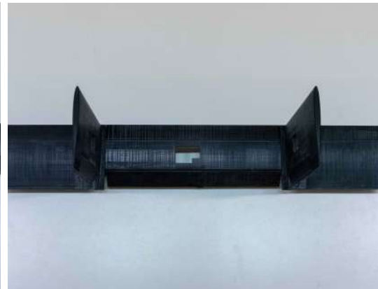
(j) Step five: insert and screw vertical tail assembly and external horizontal stabilizer in the already assembled tail (continued).
