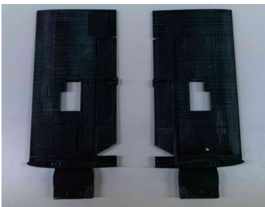
(e) Step two: screw the vertical tail to the tail-boom support piece (continued).
