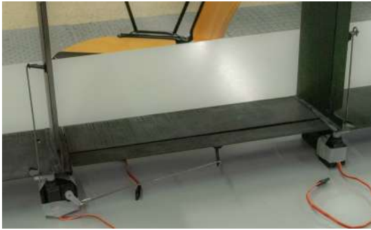
Figure 5.11: Test of the original control mechanism for rudders and elevator.
