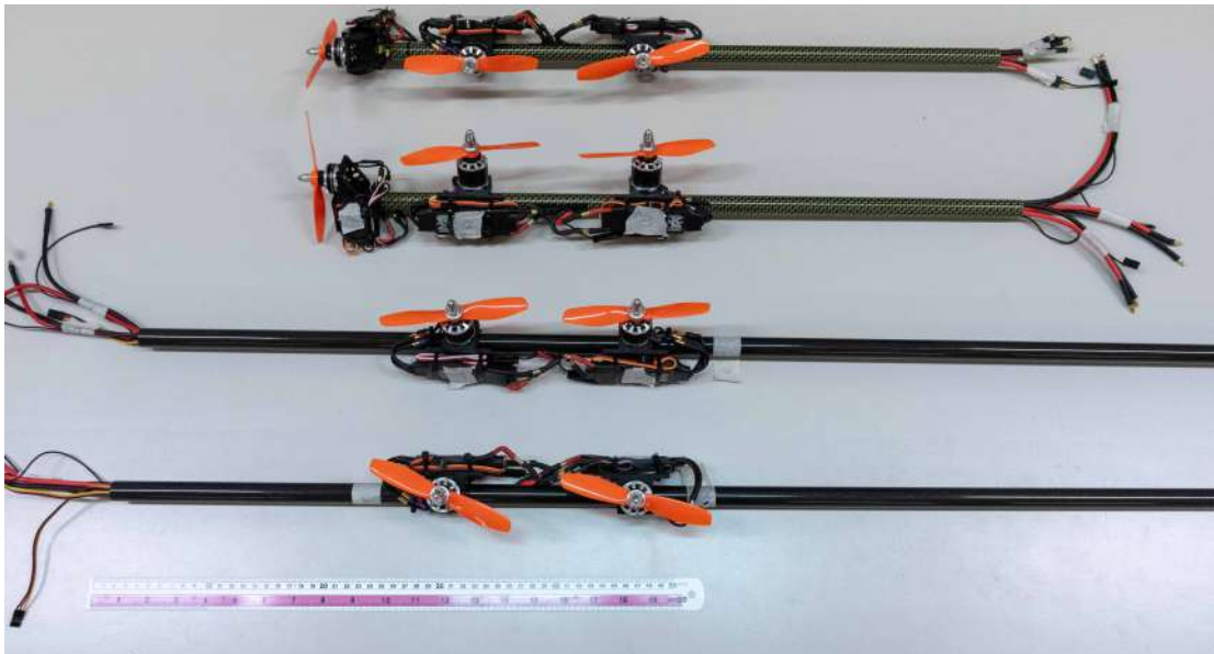
Figure 5.25: Completed motor booms, ready to be installed.
