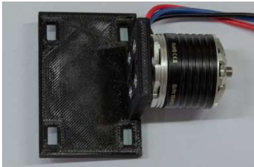
(c) Step one: mount motor on ESC plate (continued).
