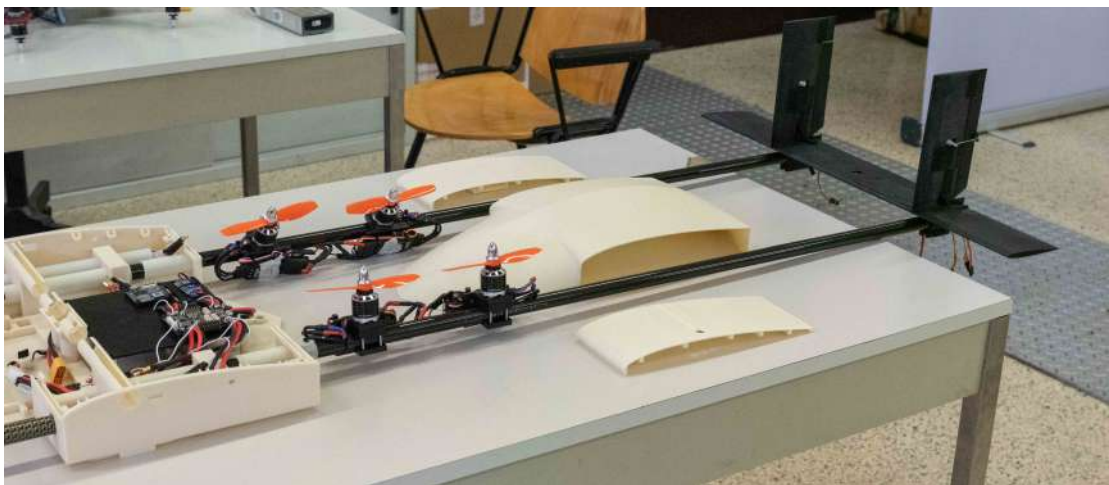
(c) Step two: insert and secure tail on rear booms.
