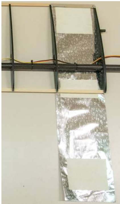
(a) Step one: apply Mylar cladding on one side of the wing.
