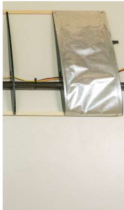
(b) Step two: wrap the Mylar cladding around the wing.
