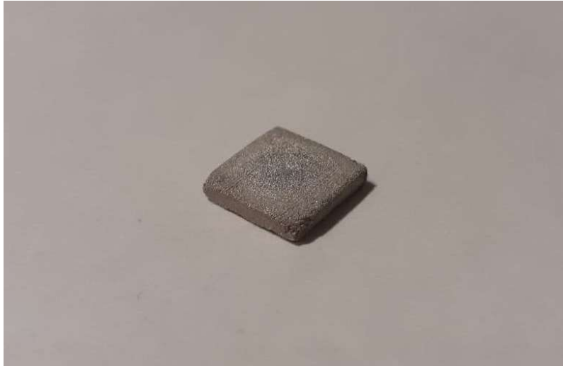
Figure 6 – 2 nd type specimen for corrosion test
