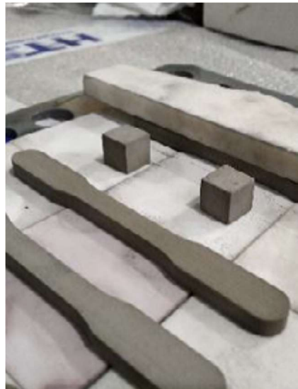
Figure 5 – 1st type specimens for tensile testing.
