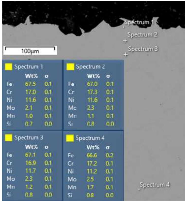
Figure 25 – SEM image of BJ CS, with EDX analysis of composition at different depths.
