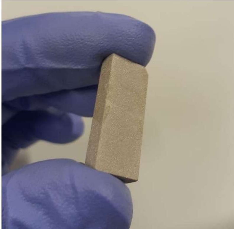
Figure 7 – Type two specimen for corrosion test
