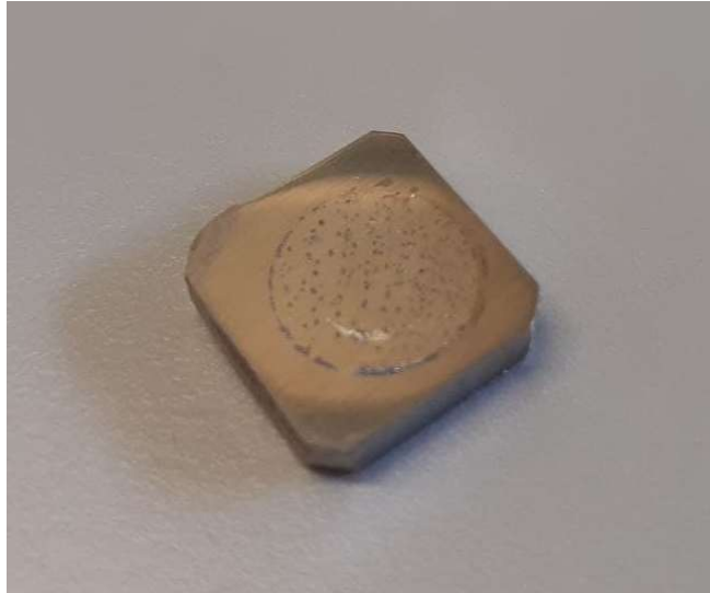
Figure 8 - specimen after the test, showing intended pitting on the exposed area.
