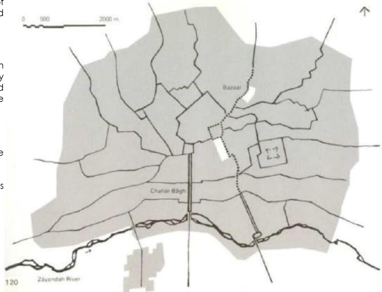
Figure1-30; Schematic map of Isfahan's water channel (Madi) system, the Maddies made an organic design in the city
