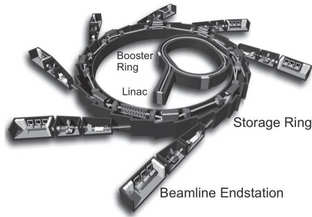
Figure 1.2: Schematic picture of a synchrotron facility [7].
