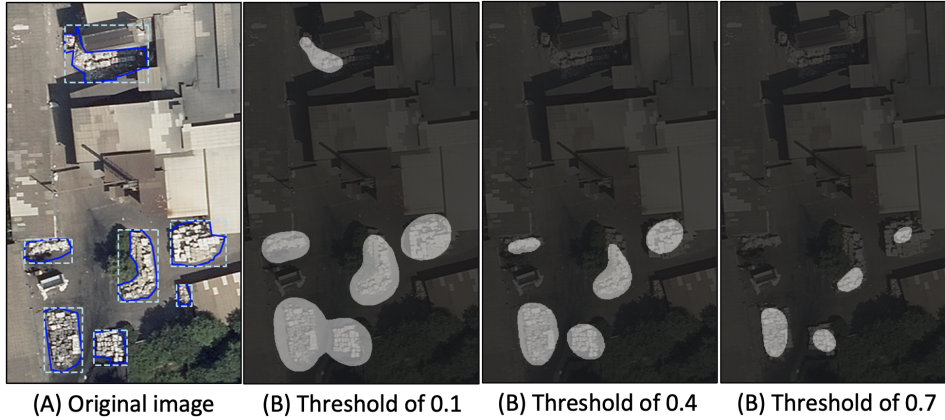
Figure 7.1: Effects of the variation of the threshold on the generated CAM mask (light grey foreground areas).
