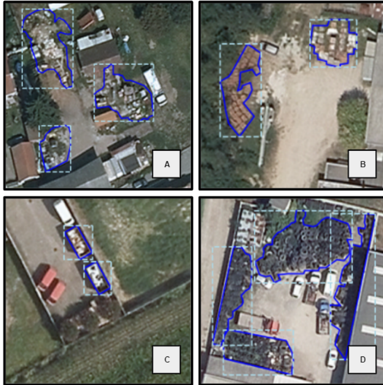
Figure 4.3: Segmentations in blue, bounding boxes in light blue. A are scattered wastes, B pallets, C dumpsters, and D tires.
