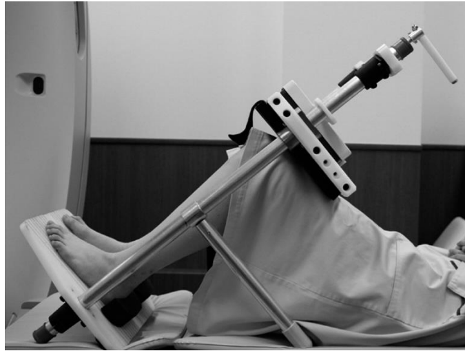
Figure 12 Example of simulated loading in standard CT. The load applied is proportional to the distance between the foot plate and the knee plate. With this mechanism the simulated load is different from the real body weight. Moreover, the apparatus is customized, so the procedure is hardly repeatable [kido et al., 2011]
