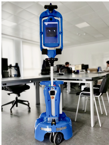
Figure 3.7: Giraff-X socially assistive robot, developed for the MoveCare project [107]
