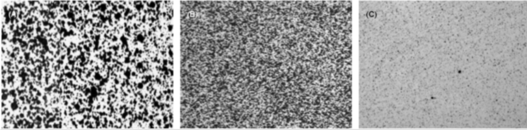
Figure 3.10: Different speckle pattern densities in the undeformed images [52].
