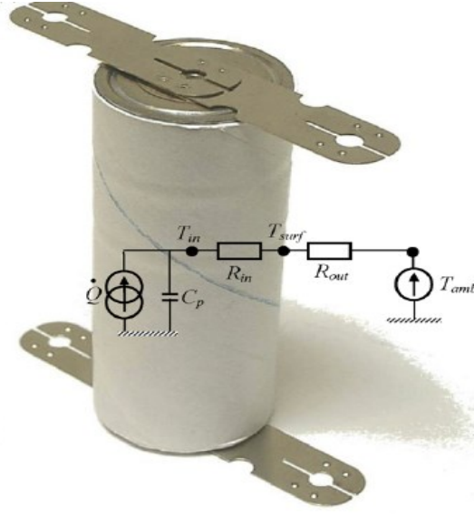
Figure 15: Battery cell's simplified thermal equivalent circuit. [30]
