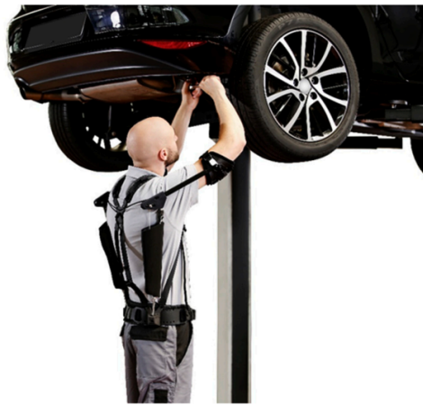
Figure 3.7: The passive exoskeleton PAEXO used in industrial environment [98].
