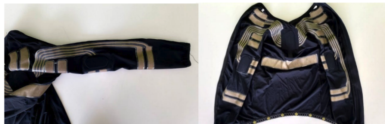
Figure 3.5: Sensors inside the Myontec Shirt. One of the arms (left) and the whole shirt (right) [92].
