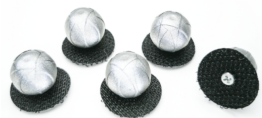
(a) Reflective markers for optical capture of movement, with circular velcro base.
