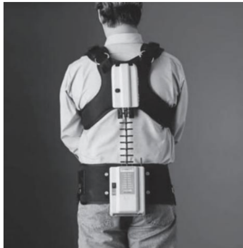
Figure 3.3: the industrial Lumbar Motion Monitor (LMM). Photo courtesy of Biodynamic Solutions, Inc.
