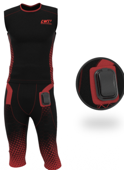
Figure 5.1: WINGS wearable components. Left: sensorized Shirt and Shorts. Right: wireless data processing and transmittance system embedded into the shirt and shorts.
