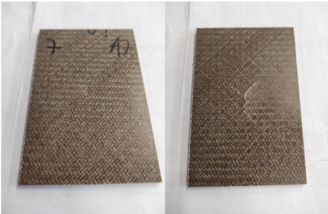
Figure A.13: Indentation test specimen 7
