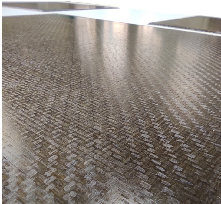
Figure 4.1: Detail of an ampliTex™ 300 laminate
