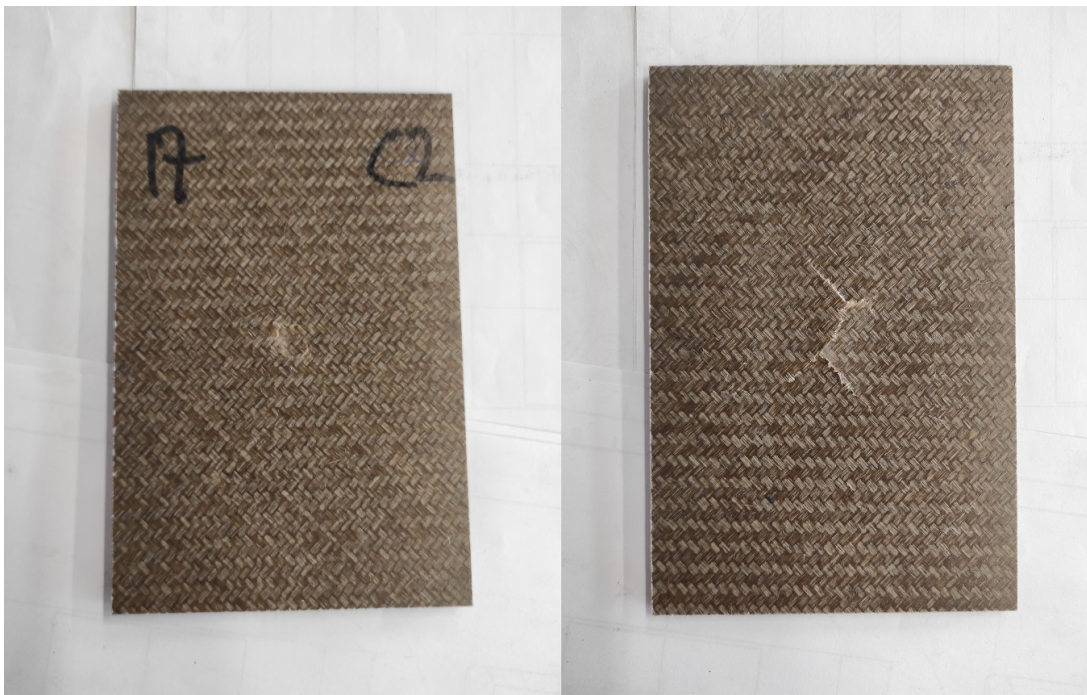
Figure A.17: Indentation test specimen 17
