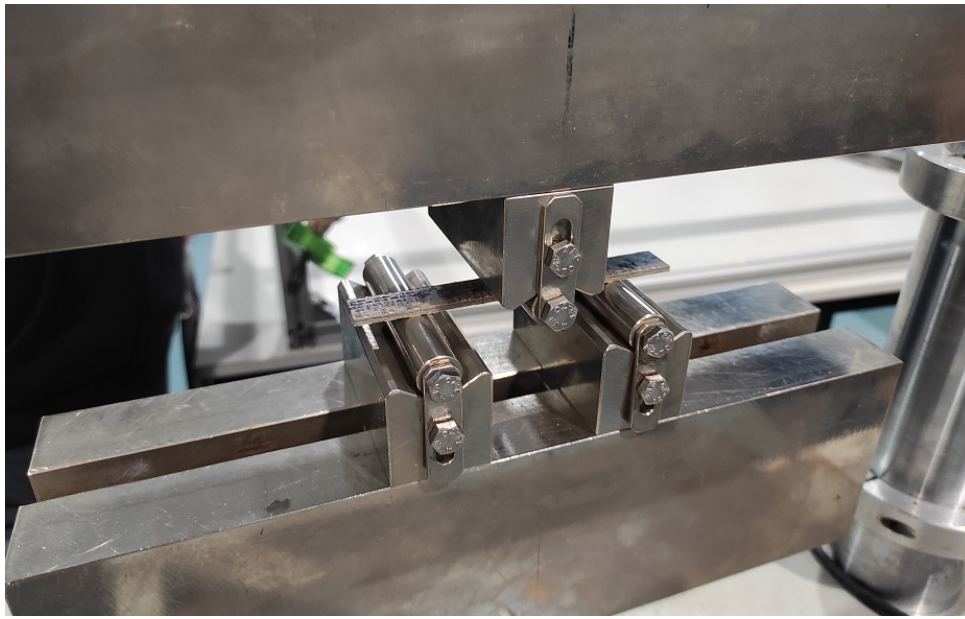
Figure 4.13: Bending test set-up
