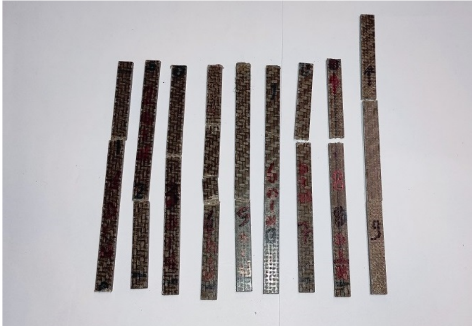
Figure A.8: Strain rate test specimens without strain gages
