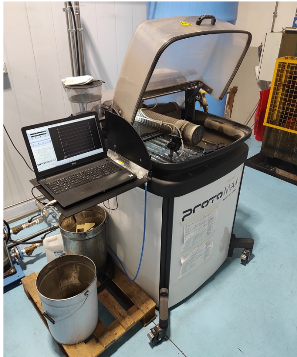
Figure 4.4: ProtoMAX abrasive waterjet cutter
