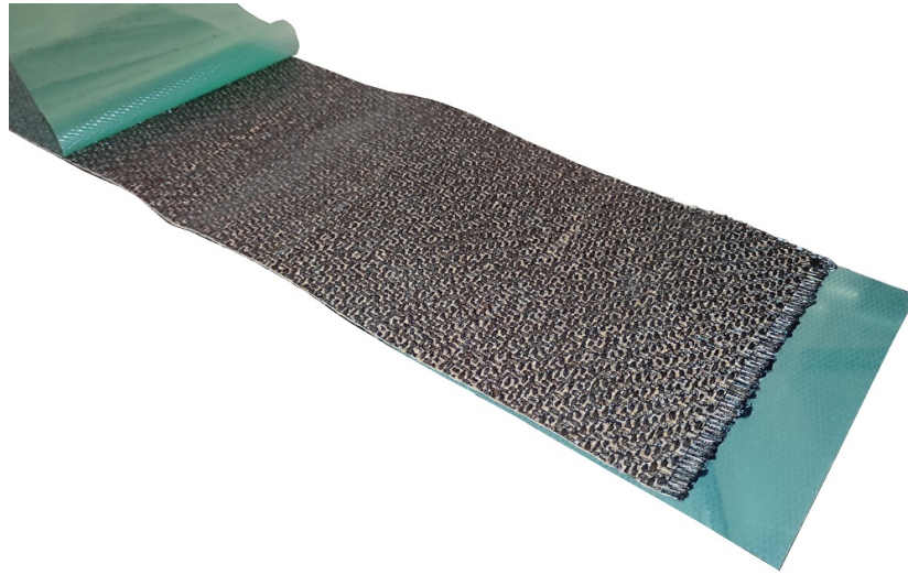
Figure 2.23: Sample of prepreg lamina
