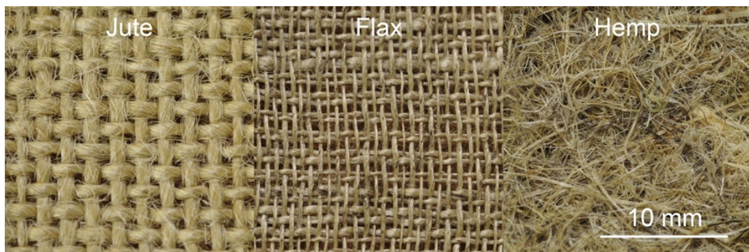
Figure 3.6: Macroscopic detail for each fiber type
