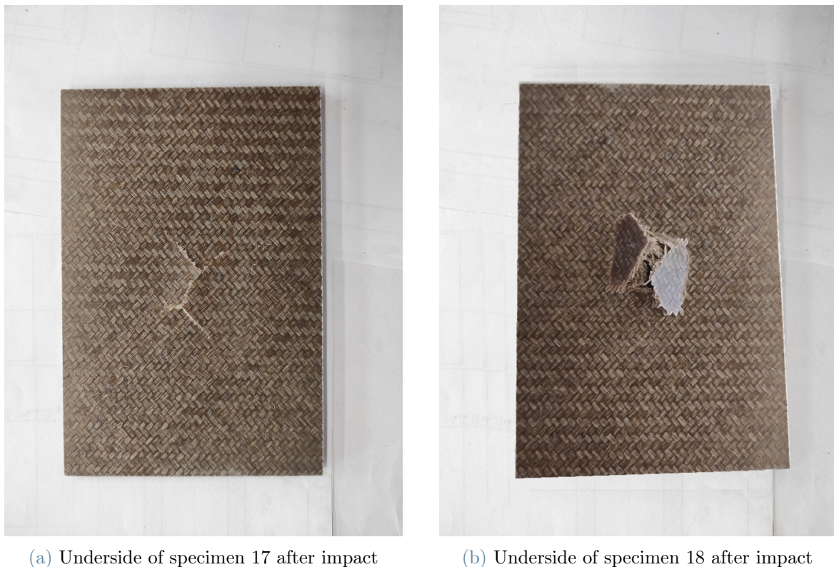
Figure 4.32: Representative failure modes indentation test
