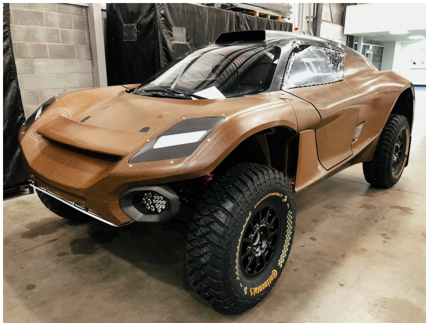
Figure 3.4: Abt Cupra XE body shell made of flax composite materials
