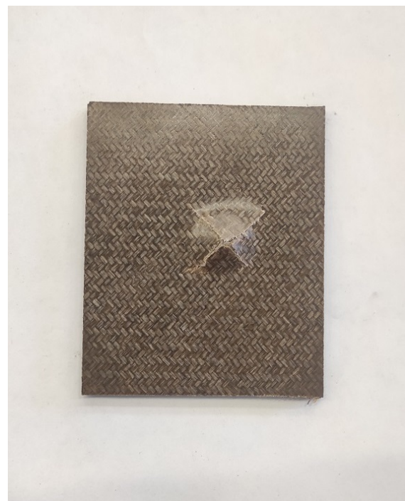
(b) Underside of specimen 8 after impact
