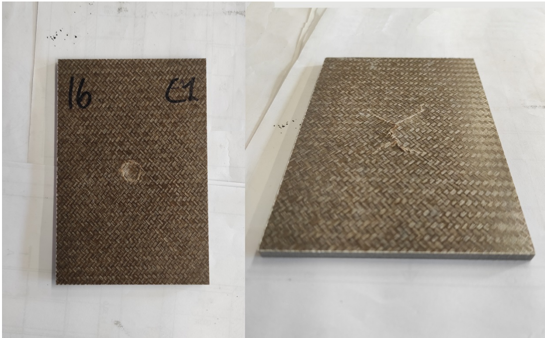
Figure A.16: Indentation test specimen 16
