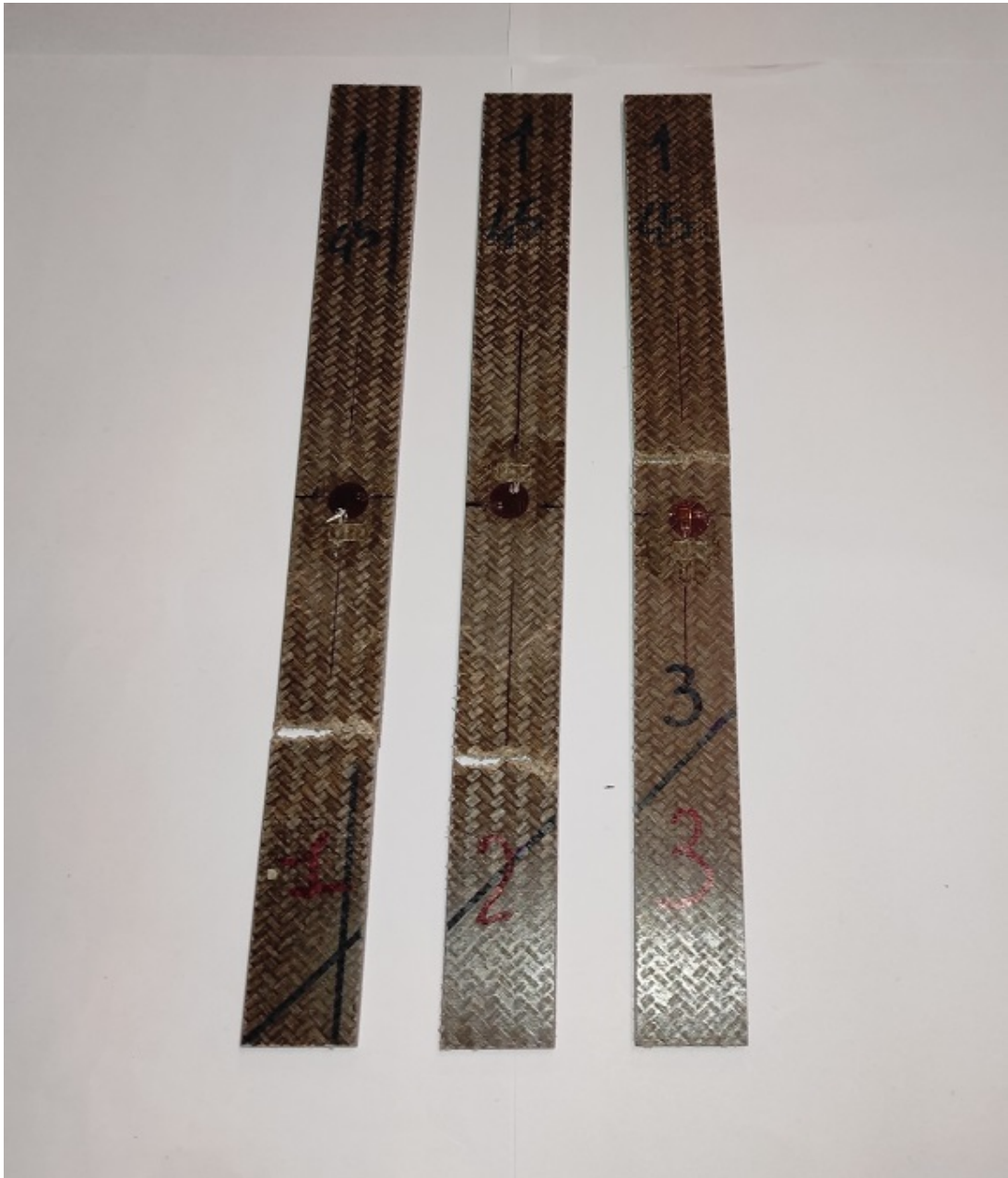
Figure A.3: Shear test specimens
