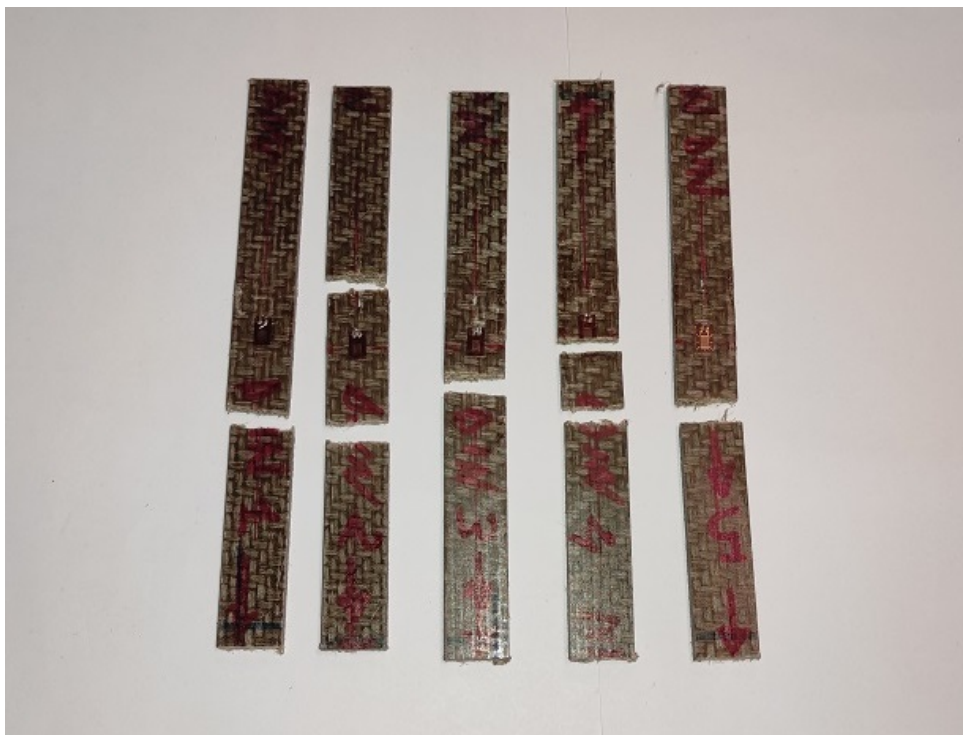
Figure A.9: Strain rate test specimens equipped with strain gages
