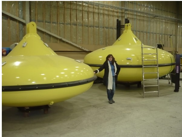
Figure 1.4: Point absorbers in the Lysekil's factory.
