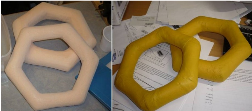
Figure 3.8: Polystyrene before and after the application of the fiberglass.
