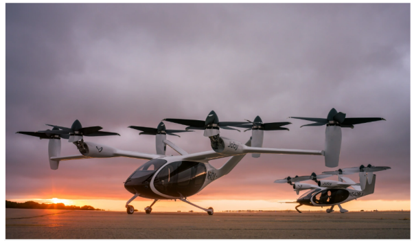
(b) eVTOL of Joby aircraft in take off and landing configuration.
