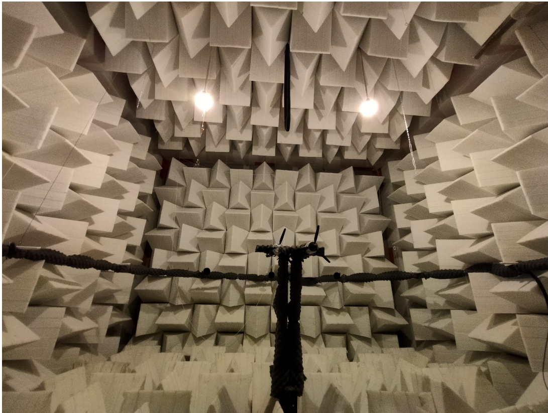
Figure 2.6: View of the anechoic chamber in a completely anechoic setup.
