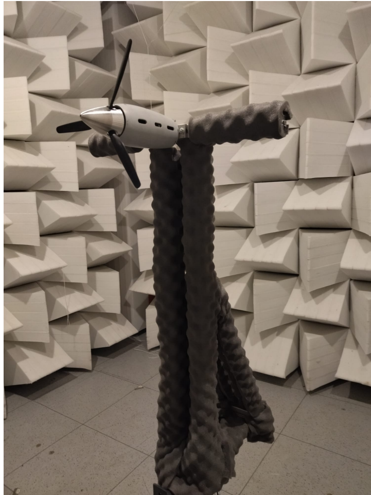
Figure 2.3: Bosch © structure on which a single propeller is mounted.
