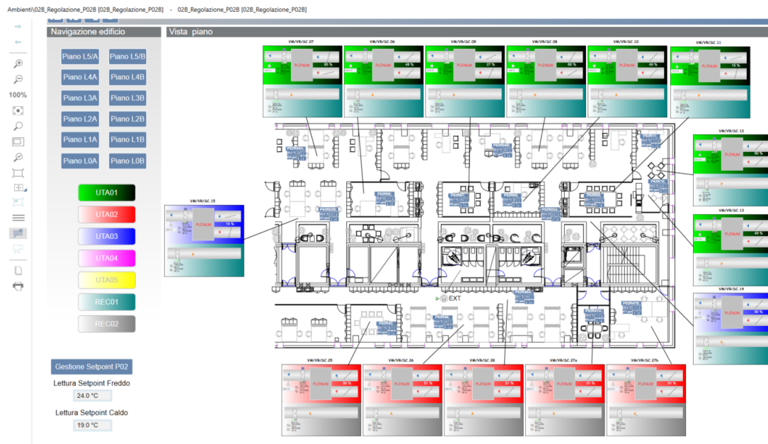
Figure 3.11: Floor control interface
