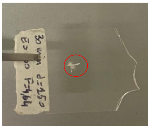
Figure 4. 4 Picture of the glass with the clear damage caused by the laser.
