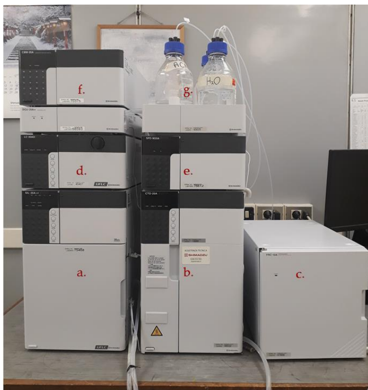
Figure 3. 5 HPLC apparatus employed in this work: the autosampler (a); oven and columns (b); the fraction collector (c); the pump system (d); the photodiode array spectrometer (e); the controller (f); solvent tray (g)
