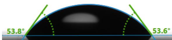
Figure 4.14: A picture of the drop shape with its relative contact angle of a sample silanized with VPD protocol.
