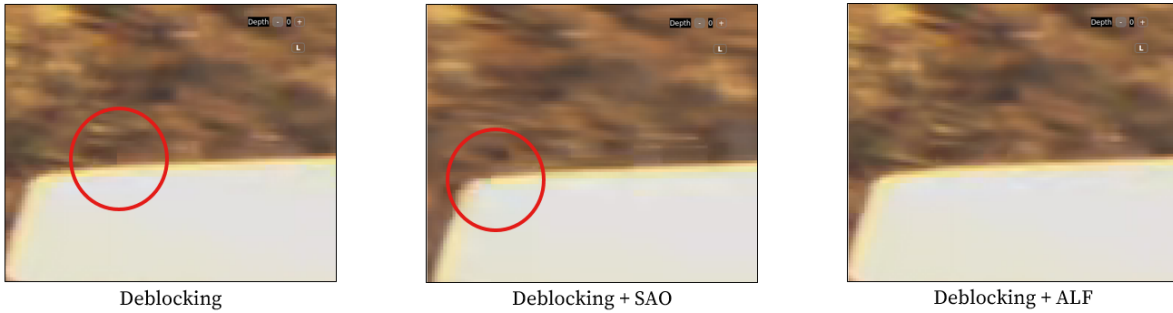
Figure 1.3: Apparent defects in a reconstructed image then filtered by different In-Loop Filters.
