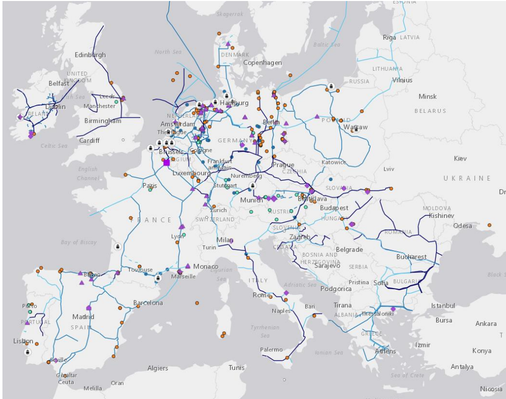
Figure 1.3: Expected European Hydrogen Infrastructure map in 2040. Darkest lines are existing reconverted pipelines, light blue new pipes and dark blue a mix of both. [7]
