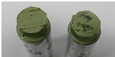
Figure 1.1: Adhesive failure Figure 1.2: Cohesive failure Figure 1.3: Mixed failure
