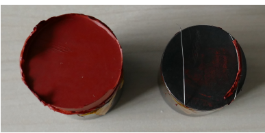
Figure 1.1: Adhesive failure Figure 1.2: Cohesive failure Figure 1.3: Mixed failure
