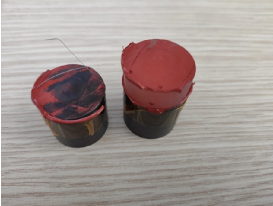
Figure 4.9: Adhesive failure in RTV566
