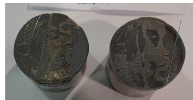
Figure 1.1: Adhesive failure Figure 1.2: Cohesive failure Figure 1.3: Mixed failure
