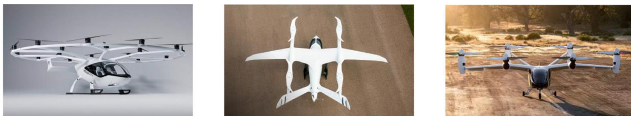
Figure 7. Prominent examples of different eVTOL configurations: VoloCity (left), Beta ALIA-250 (centre) and Joby S4 (right)
