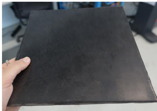
Figure 3.10: Shot fiber autoclave processed panel
