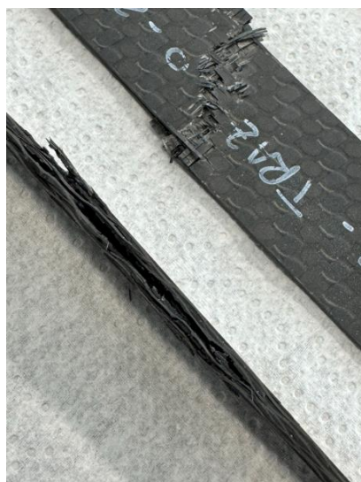
Figure 4.16: C630 TR50 IMP512 delaminated tensile sample
