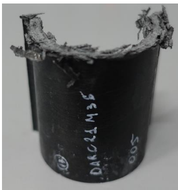
Figure 4.76: Pulverized C200 Carbon Task IMP509's omega samples
