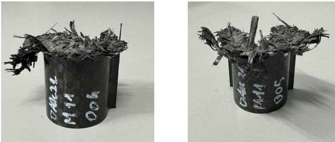
Figure 4.11: Petal failure of C370 MR60 IMP512's omega samples
