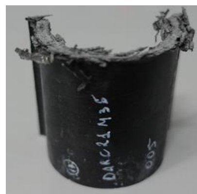
Figure 4.111: C200 Carbon Task IMP509 omega sample
