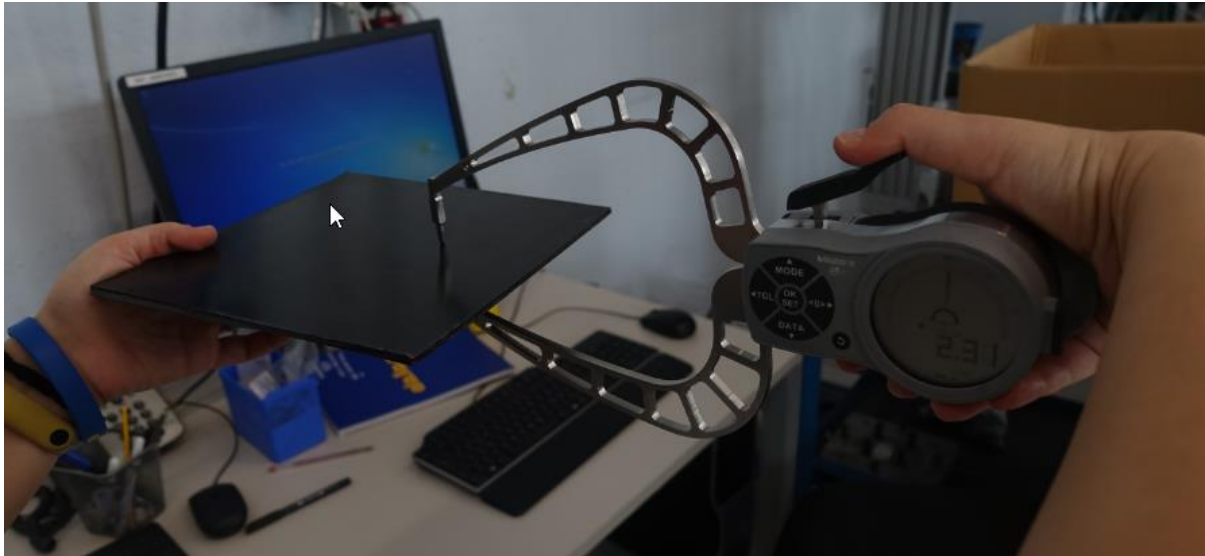
Figure 3.23: Thickness measuring of autoclave processed panel
