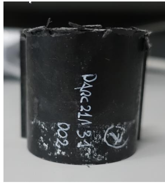
Figure 4.53: Pulverized C200 Carbon Task IMP512's omega samples
