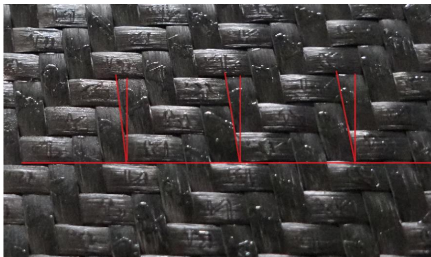
Figure 4.1: Fiber misalignment of C630 TR50 12K IMP512 BIO
