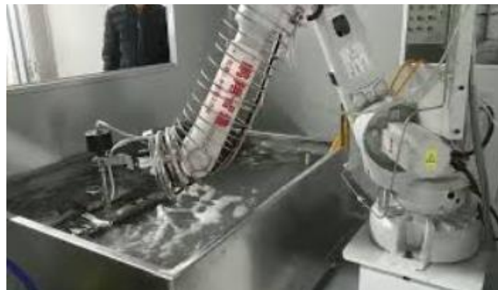
Figure 3.28: Example of waterjet robotic arm
