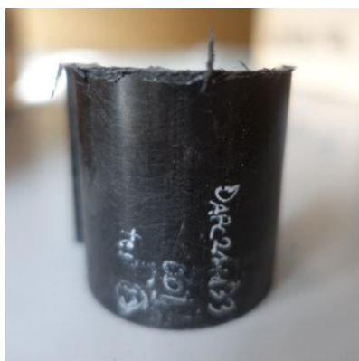
Figure 4.78: Pulverized C100 Carbon Task IMP512's omega samples
