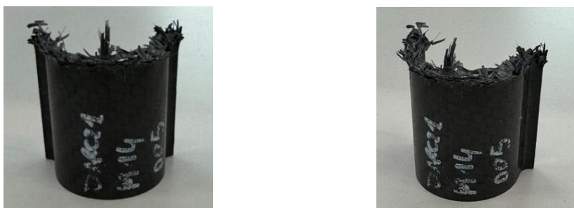
Figure 4.24: Hybrid failure of C630 TR50 IMP512's omega samples
