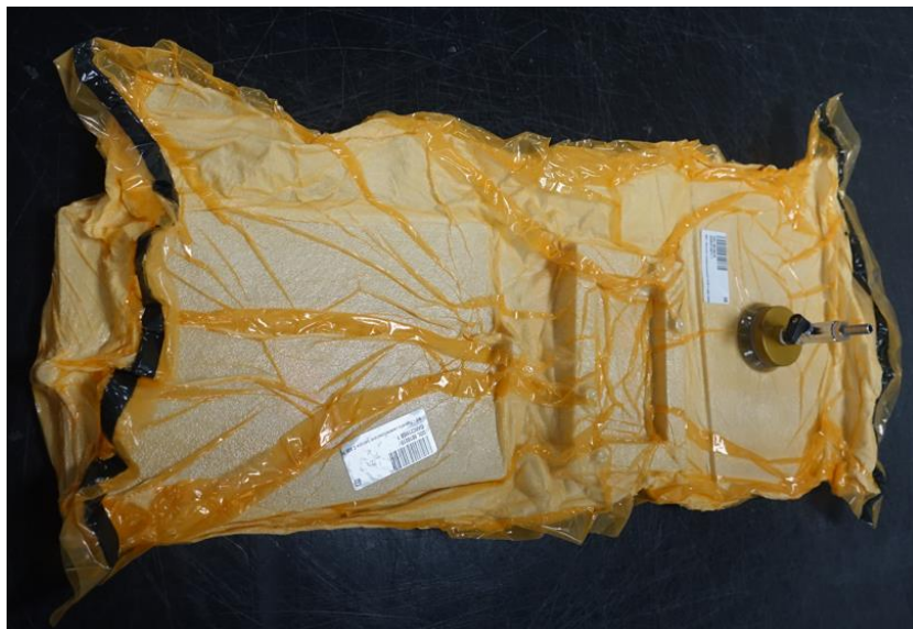
Figure 3.3: Vacuum bag with Vac valve
