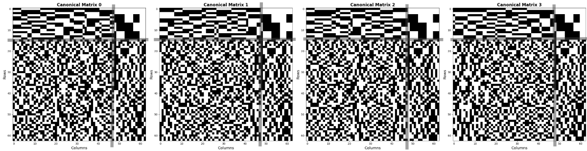
Figure 7.5: Reordered forms of neos5 obtained by applying GCG decomposition, block ordering, and recursive rules
