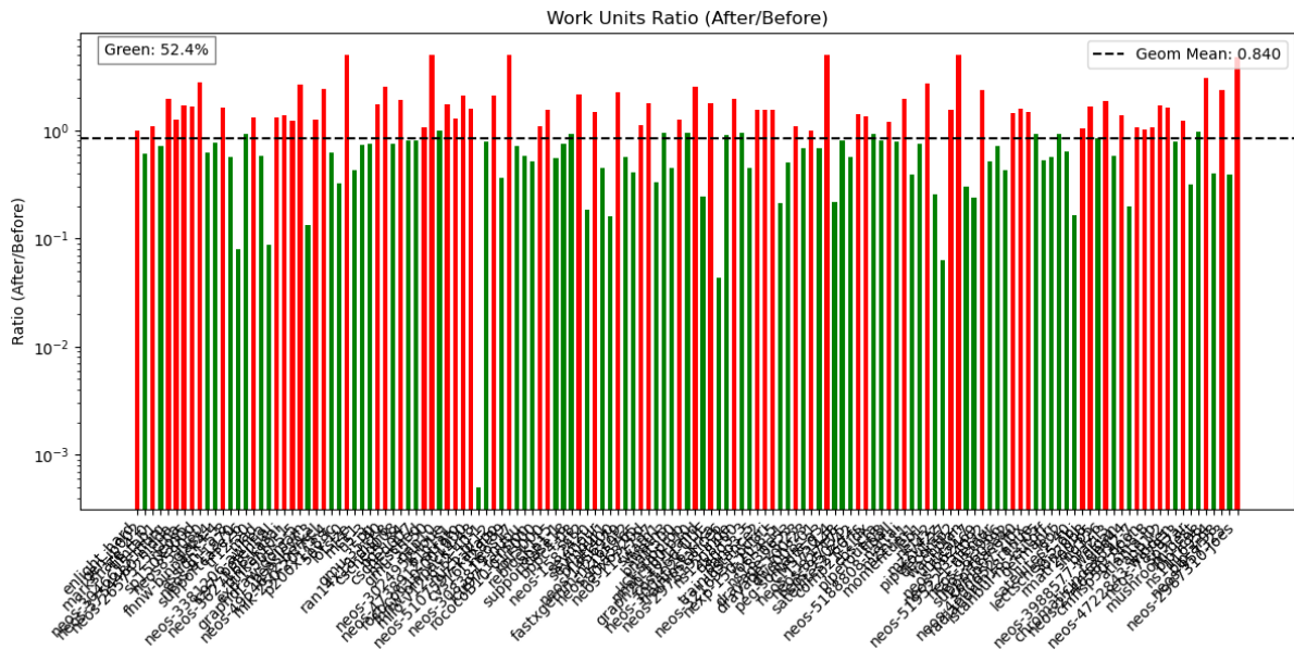
Figure 7.2: Work units ratio comparing original and reordered problems after applying both GCG decomposition and block ordering rules. Ratios below one indicate a reduction in runtime variability, suggesting that combining decomposition with block ordering improves the consistency of solver performance. The percentage of instances with reduced variability is shown at the top left, and the geometric mean of the ratios is shown at the top right
