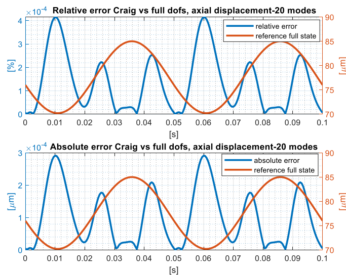
Figure 6.1: Craig reduction (20 modes) compared to complete model considered as reference, in terms of relative error (above) and absolute error (below) of axial displacement
