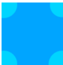
Figure 3.2: Aspect of a sample after deposition of Parylene. On the corner the color is less blueshift due to the lower ratio between bromide and chlorine ions.
