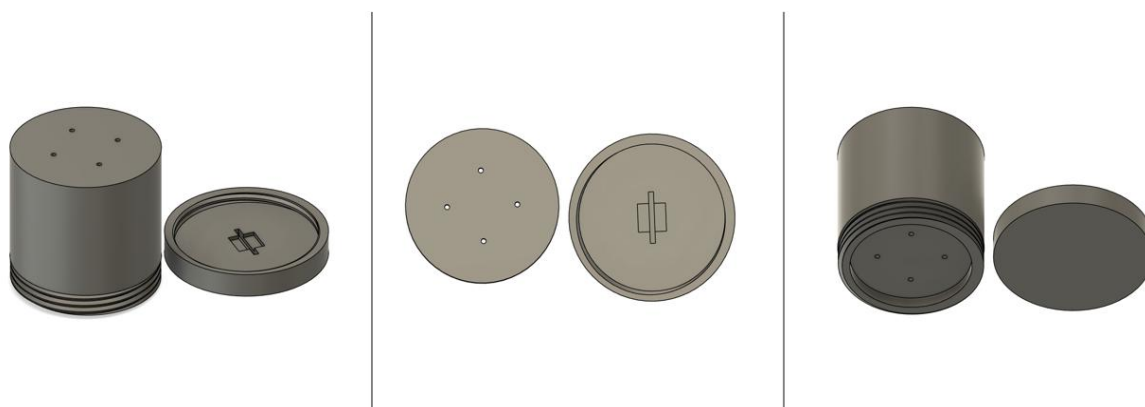
Figure 3.7: 3D models of the flux limiter with 4 channels of 60 mm length. The holder is designed for 1 cm 2 substrates
