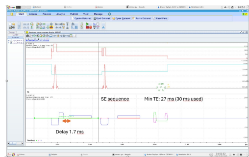
(b) PGSE obtained from the free gradient waveform interface with single-line SE readout.
