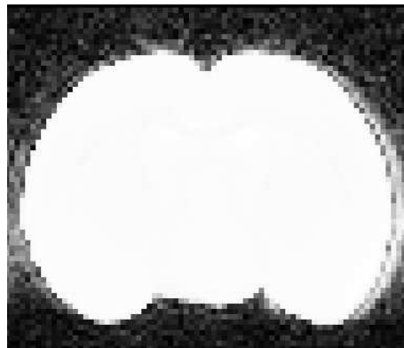
Figure 5.9: Nyquist ghost artifact observed before double sampling was implemented. Note that the contrast was increased.
