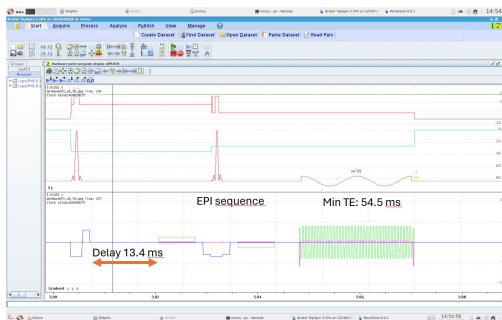
(a) PGSE obtained from the free gradient waveform interface with single-shot EPI readout.
