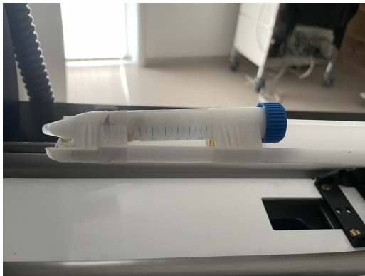
Figure 4.2: Side view of the sample mounted on the MRI bed. Note the slight slope to avoid air bubbles in the area of interest.
