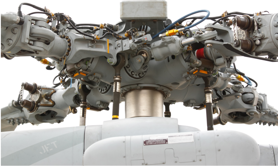
Figure 1.2: Four-blade rotor with blade-to-hub arrangement of a Sikorsky MH-60 helicopter, source in [10].
